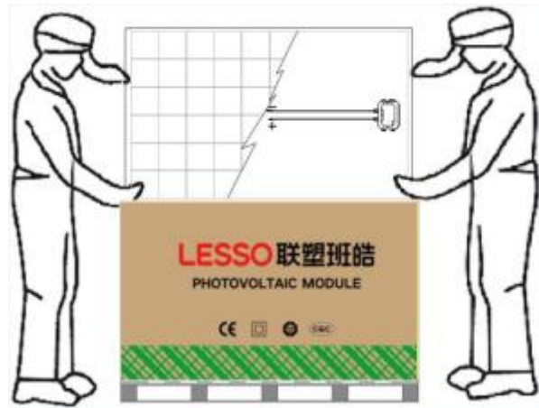
Figure 2 Removing PV modules from a pallet
